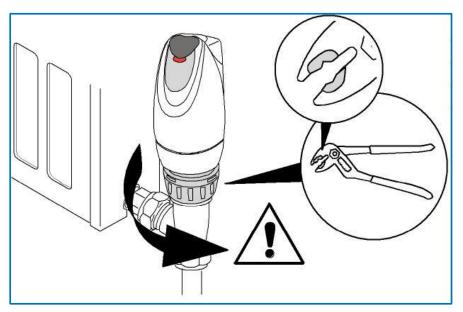
To remove the eTRV, use wide jaw plumbing pliers.
