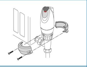
To remove the Security Thread Lock, rotate the collar so that the screws are facing you.
