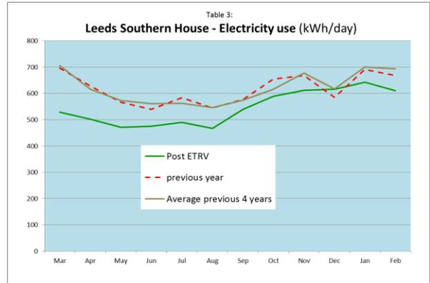
It was then realised that the power saving was from staff no longer using portable electric heaters to enhance individual local comfort, with these no longer in use, the gas fired heating filled the gap. With electricity being up to 4 times the cost of the gas, the power financial savings boosted overall project performance to actually exceed expectations by 18%.
