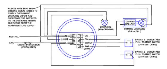
**NOTE** - The center biased retractive switch is an optional feature. If the switch is not required, the controller is fully automatic based on occupancy.
