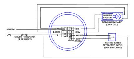
**NOTE** - The center biased retractive switch is an optional feature. If the switch is not required, the controller is fully automatic based on occupancy.
