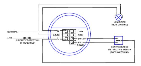
**NOTE** - The center biased retractive switch is an optional feature. If the switch is not required, the controller is fully automatic based on occupancy.
