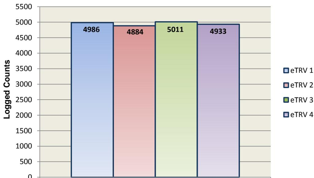
Graph 4.0: Complete travels made before power loss
