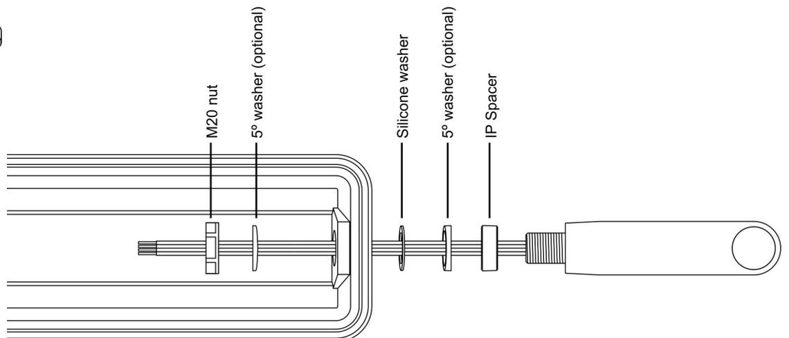
*Note. Use the 5° spacers where the luminaire housing has a draft angle.*
